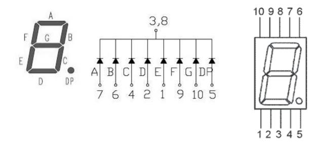
The displays have a common cathode pin meaning you hook that pin to your 330 ohm resistor which in turn is hooked to ground. The anode pins of the display go to various digital I/O pins.
