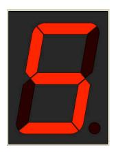
I have a few 7-segment displays I can loan out. These are fairly simple to hook up to the Arduino. The displays have a common cathode pin meaning you hook that pin to your 330 ohm resistor which in turn is hooked to ground. The anode pins of the display go to various digital I/O pins.
